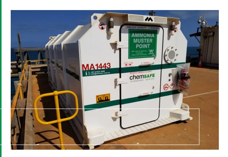
Pictured Right: A 12-Person customised MineARC ChemSAFE Standard Design Safe Haven.
