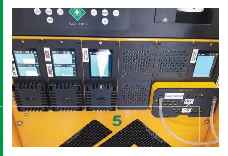
Pictured: Aura-FX Internal and External Digital Gas Monitoring
