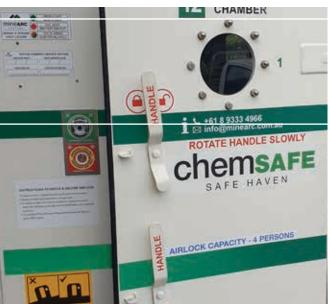
As the safe haven serves as an emergency chemical shelter and command centre, safety and operations personnel must be able to enter and exit the chamber multiple times during an emergency.
