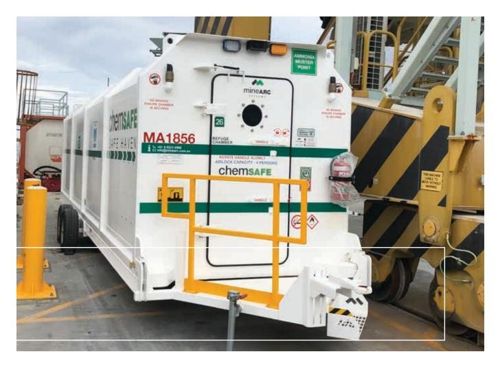
Pictured: Wheel and Tow additional helps transport the refuge on and off the wharf
